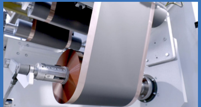
Above: Flexible rotational direction of the unwinding unit
