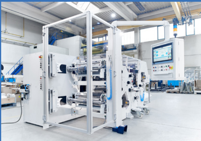
Above: Flexible rotational direction of the unwinding unit
